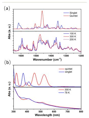
Fig. 4 Experimental and calculated temperature-dependent IR and UV spectra of complex 2.0.5EtOH. (a) Calculated IR absorption for singlet and quintet states (upper), and temperature-dependent IR spectra recorded between 100 and 300 K (lower). (b) Calculated UV absorption spectra for singlet and quintet states (upper), and temperature-dependent UV spectra recorded between 78 and 300 K (lower).
