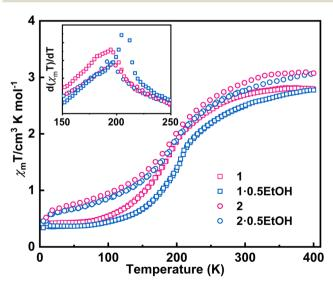
Fig. 2 Magnetic properties of complexes 1 and 2. The temperaturedependent magnetic susceptibility was performed at a sweeping rate of 5 K min<sup>-1</sup>. The magnetic susceptibilities of compounds 1 and 2 are shown by open squares and circles, respectively. Magnetic properties before and after desolvation are marked in red and blue, respectively. Inset: First-order derivatives of the  $\chi_{\rm m}T$  product in the cooling process.
