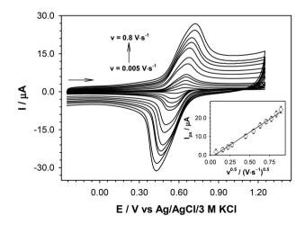
Fig. 3 Cyclic voltammograms of compound 4 recorded in DCM with the addition of tetrabutylammonium hexafluorophosphate (TBAPF<sub>6</sub>). Inset: Dependencies of anodic peak current vs. square root of scan rate. Experimental conditions:  $C_{compound} 4 = 0.1 \text{ mM}$ ,  $C_{TBAPF_6} = 50 \text{ mM}$ , glassy carbon disk electrode ( $\emptyset$  = 3 mm); T = 21 °C.
