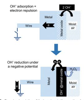
Fig. 15 Stepwise description of the two steps in the negative electrode of a hygroelectric cell: (top) adsorption: an isolated electroneutral acidic oxide surface in contact with moisture adsorbs OH- ions acquiring negative charge. (bottom) Redox reaction: electron transfer from OHions to the electrode produces hydrogen peroxide. Adapted with permission from ref. 131. Copyright 2023. American Chemical Society.
