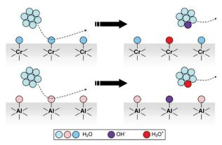
Fig. 7 Schematic description of metal charging under a moist atmosphere. Aluminum metal is always coated by an acidic oxide layer that picks hydroxide ions from impinging water clusters, acquiring negative charge. Stainless steel and other alloys contain basic chromium oxide and bind hydronium ions from atmospheric water, acquiring positive charge. Reproduced with permission from ref. 32. Copyright 2023. American Chemical Society.
