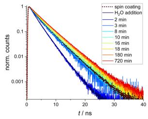
Fig. 2 Normalized TCSPC decay curves obtained from the FLIM images measured directly after spin coating (dotted black line), after addition of H<sub>2</sub>O (dark blue line) and after different drying times, respectively. For bi-exponential fits and residuals see the ESI.†
