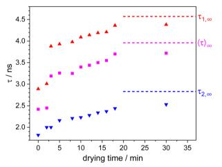
Fig. 3 Fluorescence lifetimes  $\tau_1$  and  $\tau_2$  fitted with a bi-exponential fit and amplitude-weighted average fluorescence lifetimes  $\langle \tau \rangle$  for different drying times after addition of a  $\approx 10~\mu L$  drop of water to spin-coated microgels. The dashed lines represent the fluorescence lifetime values obtained by a fit of the TCSPC curve measured after 720 min (overnight) drying time.
