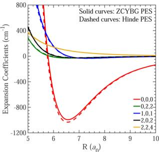
Fig. 1 The dominant expansion terms in the angular dependence of the HD-D<sub>2</sub> PESs as a function of the intermolecular separation. The solid curves represent the results from the ZCYBG PES, 23 while dashed curves are obtained using the Hinde PES.<sup>22</sup> The numbers in the legends correspond to  $\lambda_1$ ,  $\lambda_2$ , and  $\lambda_{12}$ , respectively.
