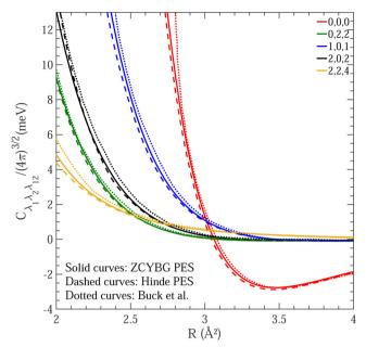
Fig. 2 Same as Fig. 1. In addition to the solid curves obtained from the ZCYBG PES<sup>23</sup> and dashed curves from the Hinde PES,<sup>22</sup> the dotted curves show available results using the M80 PES reported by Buck et al. 76 Note the different units for the energy and R compared to Fig. 1.
