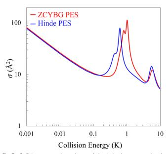
Fig. 7 Collision energy dependence of the inelastic cross section for  $\Delta j_{HD} = -1$  transition in HD( $v_{HD} = 1$ ). The blue and red curves represent results obtained on the Hinde and ZCYBG PESs, respectively.
