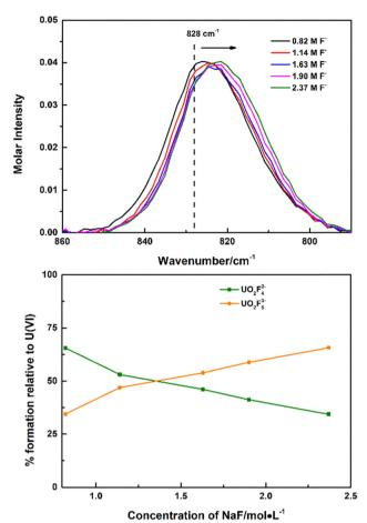
Fig. 2 Raman spectra of UO<sub>2</sub>(NO<sub>3</sub>)<sub>2</sub> in 2.5 M (CH<sub>3</sub>)<sub>4</sub>NNO<sub>3</sub>/(CH<sub>3</sub>)<sub>4</sub>NNO<sub>3</sub> (top) and speciation distribution during titration (bottom).  $C_{uranvl} = 0.059$ M,  $C_{\text{pitrate}} = 0.118 - 1.69 \text{ M}$ , V = 1.0 mL,  $C_{\text{H}}^{+} = 0.002 \text{ M}$ ,  $C_{\text{fluoride}} = 0.82 -$
