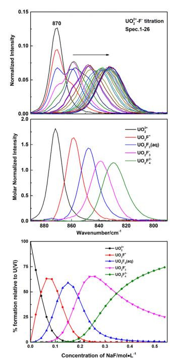
Fig. 1 Representative Raman spectral titration of U(vi) with fluoride. Top: Spectra collected during a titration (normalized to the intensity of 0.257 M perchlorate). Middle: Raman spectra of U(vi)/fluoride complexes of relative intensity from deconvolution.  $C_{\text{uranyl}} = 0.074 \text{ M}$ ,  $C_{\text{perchlorate}} = 0.257 \text{ M}$ , V =0.66 mL,  $C_{H}^{+}$  = 0.003 M,  $C_{fluoride}$  = 0-0.54 M. Bottom: Speciation distribution during the titration.
