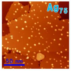
Fig. 1 STM image of soft-landed Ag $_{75}$  NCs on a C $_{60}$  substrate (160 imes160 nm²) at a low coverage (  $\sim\!4\times10^3$  dots per  $\mu m^2\approx7.3\times10^{-3}$  ML). The tip bias voltage ( $V_t$ ) and tunneling current ( $I_t$ ) are  $V_t = -2.0$  V and  $I_t = 10$  pA, respectively. Bright dots correspond to individual Ag<sub>75</sub> NCs, monodispersively immobilized on the  $C_{60}$  surface, where the average height of  $Ag_{75}$
