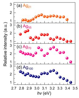
Fig. 5 Photon energy dependence of photoemission in  $Aq_n/C_{60}$  (n = 21, 55, 70, and 100), measured with s-polarized light within the range of 2.77 to 3.45 eV. Above n = 70, photoemission enhancements with s-polarized light are observed, resulting in a decrease in  $I_p/I_s$  values.
