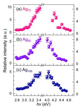
Fig. 4 PIE intensities integrated from  $E_{\rm F}$  + 2hv to  $E_{\rm F}$  + 2hv - 0.5 eV for three sizes of  $Ag_n$  NCs (n = 70, 85, and 100) against hv in p-polarization. The peak of PIE intensities could not be observed with the  $h\nu$  window of the SH and TH photons in this study
