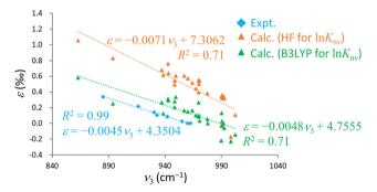
Fig. 4 Relationships between  $\nu_3$  and  $\varepsilon$ . The horizontal axis shows  $\nu_3$  in units of cm $^{-1}$  while the vertical axis shows  $\varepsilon$  in units of %. The dotted lines are linear regressions and  $r^2$  is the coefficient of determination in each case
