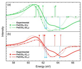
Fig. 6 Difference Fe 3p X-ray photoelectron spectra for the two lowestenergy structures of Fe(CO)<sub>3</sub> (a) and Fe(CO)<sub>4</sub> (b) simulated using MR-ADC(2)-X and compared to the experimental spectrum from ref. 15. Vertical lines represent the computed core ionization energies and the corresponding photoelectron intensities. Blue lines correspond to Fe(CO)<sub>5</sub>. No shift was applied to the simulated spectra. See Section 3 for computational details.
