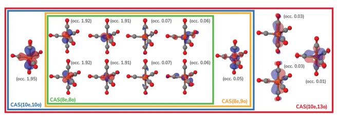
Fig. 2 Active spaces of the Fe(CO)<sub>5</sub> complex used for the multireference calculations in this work. For each orbital, natural occupations from the CAS(10e.13o) calculation are shown in parentheses
