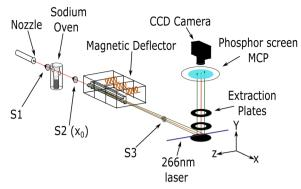
Fig. 1 Sketch of the experimental setup consisting of four vacuum chambers separated by skimmers (S1-S3). The molecular beam trajectory for deflector-off measurements is represented by a red line, while the trajectory of a spin 1/2 particle with the deflector on is depicted by green lines. For deflection measurements, S3 was removed.
