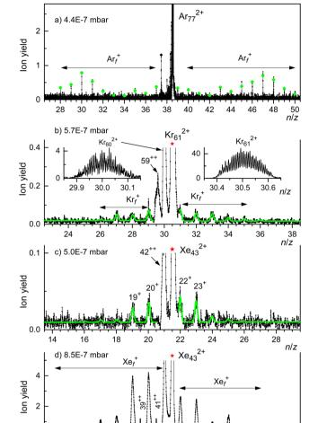
Fig. 5 Panels a through c: fragment ions produced by collisional activation of  $Ar_{77}^{2+}$ ,  $Kr_{61}^{2+}$ , and  $Xe_{43}^{2+}$  with background gas. Most of the fragment ions are singly charged except for dicationic Kr and Xe clusters that result from evaporation of one or two atoms from the precursor. The spectrum in panel d reveals a strong increase in the yield of singly charged fragments and a shift of their size distribution to the left when the collision gas pressure is increased.
