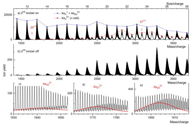
Fig. 3 Mass spectra of Xe cluster ions. Triangles and asterisks in panel a flag cluster ions for which the size-to-charge ratio n/z is integer and half-integer, respectively.  $Xe_{25}^{2+}$  is the smallest odd-numbered dicationic cluster. Panel b: no dications appear when the second ionizer is turned off. Panel c: three sections of the spectrum shown in panel a. Lines indicate the expected distribution of isotopologues of  $Xe_{25}^{2+}$ ,  $Xe_{27}^{2+}$ , and  $Xe_{29}^{2+}$
