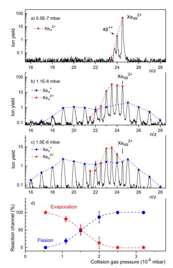
Fig. 6 Panels a through c: fragment ions resulting from collisional excitation of Xe<sub>49</sub><sup>2+</sup> recorded with increasing collision gas pressure. Contributions from singly and doubly charged ions to the mass peaks are indicated by dots and asterisks, respectively. Panel d displays the relative yield of dications (evaporation) and monocations (fission) versus collision gas pressure.
