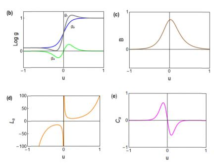
Fig. 6 (a) Equivalent circuit. Functions determining the impedance response. (b) Differential conductances,  $g_t = g_b + g_a$ . (c) B. (d) Inductor. (e) Effective low frequency capacitance. Parameters as in Fig. 4.
