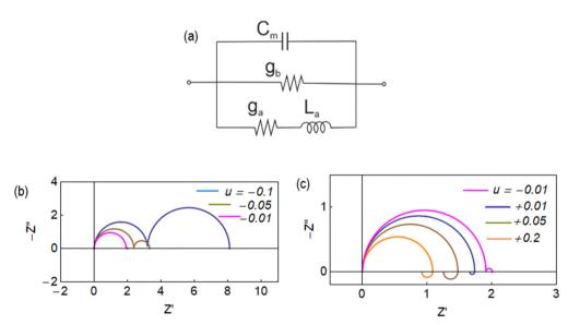
Fig. 8 (a) Equivalent circuits and (b) and (c) impedance spectra at different stationary voltages. Same parameters as in Fig. 4 and  $C_{\rm m}=0.001$ .
