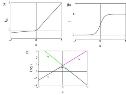
Fig. 4 (a) Current-voltage curve. (b) Equilibrium value of the state variable. (c) Relaxation times. Parameters  $V_s = 0.3$ ,  $V_r = -0.4$ ,  $V_m = 0.1$ ,  $n_s = 1.5$ ,  $n_r = 2$ ,  $g_{\rm L}$  = 0.1,  $g_{\rm H}$  = 1, and  $\tau_{\rm k}$  = 1.
