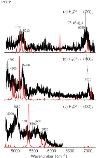
Fig. 3 Observed (black) and calculated (red) NIR spectra of  $H_3O^+\cdots(CO)_n$ , (a) n = 1, (b) n = 2, and (c) n = 3, in the OH stretching overtone region. The COloss fragmentation channel was monitored to record all the observed spectra.
