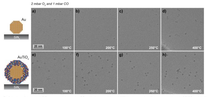
Fig. 7 Behavior of Au and AuTiO, nanoparticles under CO oxidation conditions. HRTEM micrographs of Au nanoparticles in (a)-(d) and AuTiO, nanoparticles in (e)-(h) acquired in situ at the indicated temperatures and during exposure to 1 mbar CO and 2 mbar O2. The individual images are cropped from original ones taken at different locations. Image pixel size: 0.037 nm per pixel.
