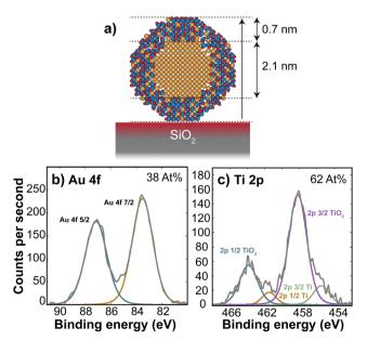
Fig. 3 XPS of the AuTiO<sub>x</sub> nanoparticles on a SiO<sub>2</sub> substrate. (a) Illustration of the estimated thickness of the shell. The XPS signal will arise mainly due to the outermost layers in the shell. (b) Au 4f and (c) Ti 2p peaks in XPS, giving an At% of Au/TiO<sub>2</sub> of 38/62 in the outer shell layers.
