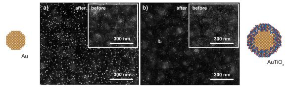
Fig. 5 Sintering after catalytic testing was observed to be more severe for the Au nanoparticles. SEM images of the (a) Au and (b) AuTiO<sub>x</sub> nanoparticles on the µ-reactors before and after reaction. All SEM images were taken with a TLD secondary electron detector with a beam acceleration voltage of 5 kV. Images pixel size: 0.68 nm (a, before), 0.62 nm (a, after), 0.83 nm (b, before), 0.62 nm (b, after). More images at different magnifications are available in ESI† Section S6
