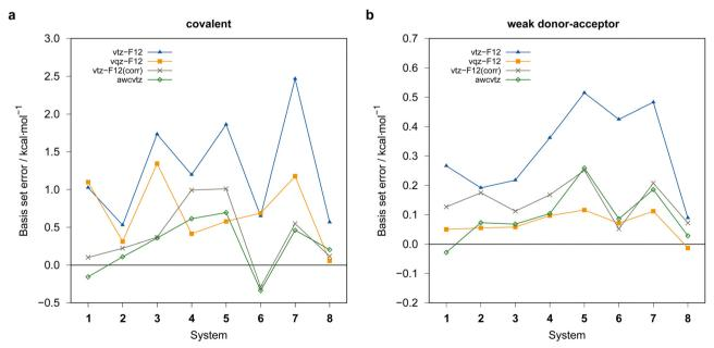
Fig. 6 PNO-LCCSD(T)-F12 basis set errors (in kcal mol<sup>-1</sup>) relative to the PNO-LCCSD(T)-F12/awcvqz reference values (using PROJECTOR=MIXED and THRPNO\_LMP2=1d-10 except for vtz-f12(corr.), see text). (a) Covalent dimers, (b) weak donor-acceptor dimers. vqz-f12 values computed with γ (opt3), otherwise  $\gamma = [1.0,1.4]$  was employed
