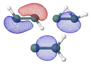
Fig. 5 Trans b<sub>u</sub>, monobridged a', and germylidene a<sub>1</sub> Ge-Ge bonding orbitals computed at HF/def2-TZVP are shown.
