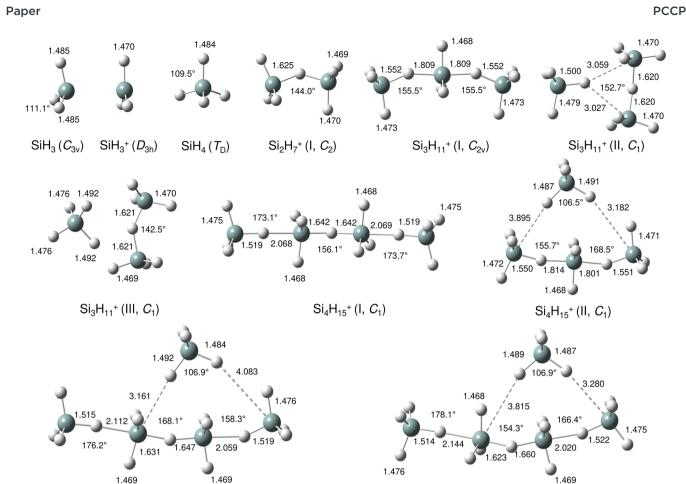
Fig. 2 Lowest energy structures of SiH<sub>3</sub>, SiH<sub>4</sub>, Si<sub>2</sub>H<sub>7</sub><sup>+</sup>, Si<sub>3</sub>H<sub>11</sub><sup>+</sup>(I-III), Si<sub>4</sub>H<sub>15</sub><sup>+</sup>(I,II) and Si<sub>5</sub>H<sub>19</sub><sup>+</sup>(I,II) in their ground electronic states calculated at the B3LYP-D3/aug-cc-pVTZ level. Selected bond lengths and bond angles are given in Å and degree, respectively.
