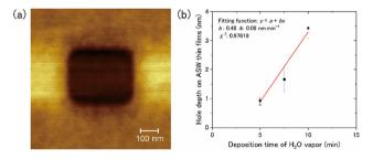
Fig. 2 (a) AFM image of a square hole made by strong tunnelling current using a scanning tunnelling microscope. (b) The relationship between hole depth and deposition time at 15 K. The red line represents the result of data fitting using a linear function.
