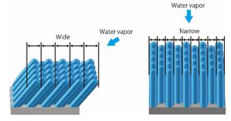
Simple morphological model of the columnar structure viewed from different directions. Arrows indicate the deposition directions of water vapor. The lateral size of surface irregularity along the y axis becomes larger than that along the x axis.
