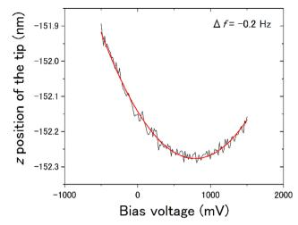
Fig. 3  $V_{\text{Bias}}$  dependence of z-positions of the tip at a single measurement point on ASW at 15 K while maintaining a constant frequency shift of  $\Delta f$  = -0.2 Hz. Lower z values indicate that the tip positions are closer to the ASW surface. The fitting function (red curve) was a guadratic function. The bias voltage at the vertex of the quadric function indicates a negative  $V_{\rm I\,CPD}$ at the measurement point
