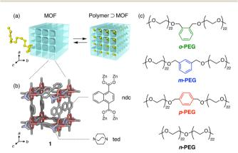
Fig. 1 (a) Schematic illustration of the nanopore threading-based polymer adsorption into a MOF. (b) Structure of MOF  $\mathbf{1}$ ,  $[Zn_2(ndc)_2ted]_n$ . The pseudo-1D channel open for polymer insertion directs to the c-axis of the MOF. (c) Chemical structures of the model PEGs possessing an ortho, meta, and para-substituted xylene moiety at the centre (o-PEG, m-PEG, and p-PEG, respectively) and non-functionalized PEG (n-PEG).
