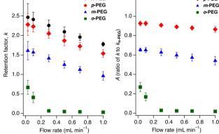
Fig. 3 Flow rate dependence of (a) k for n-PEG (black circles), p-PEG (red diamonds), m-PEG (blue triangles) and o-PEG (green squares); and (b) A  $(k/k_{n-PEG})$  for **p-PEG** (red diamonds), **m-PEG** (blue triangles), and **o-PEG** (green squares). A is a k ratio of the functionalised PEG to n-PEG. Eluent: DMF at 80 °C. The measurement conditions are identical to those employed in Fig. 2.
