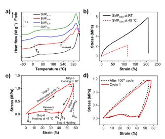
Fig. 3 (a) DSC analysis of 3D-printed SMP $_{0.33}$ , SMP $_{0.50}$ , SMP $_{0.75}$  and SMP $_{1.0}$ . (b) Tensile testing of SMP $_{0.50}$  at RT and 45 °C, (c) stress–strain plot for a thermomechanical test cycle, and (d) cyclic thermomechanical test comparison of a specimen of SMP $_{0.50}$  after 100 cycles of shape transformation cycle.
