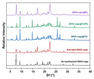
Fig. 1 PXRD patterns showing the adsorption of **Tol** and **Py** by the **DIHO-cage** after 24 h exposure.
