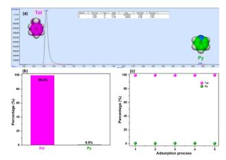
Fig. 5 (a) Relative amounts of Tol and Py adsorbed by activated DIHOcage. (b) Percentages of **Tol** and **Py** adsorbed by activated DIHO-cage as determined using GC-MS. (c) Relative uptakes of Tol and Py after each of 5 adsorption processes/cycles.
