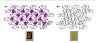
Fig. 4 Crystal packing and images of (a) DIHO-cage@Tol and (b) empty DIHO-cage@Py showing the vapochromic behaviour of DIHO-cage.
