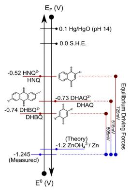
Fig. 1 Electrode potential scale showing the location of the approximate redox potentials both versus a standard reference ( $E^0$ ) and absolute electron energy  $(E_F)$ , for both the zinc/zincate couple and guinone redox couples selected as mediators. Equilibrium overpotentials between the liquid/solid components are indicated on the right-hand side. Please see ESI† for complete compound names and discussion of reactions.
