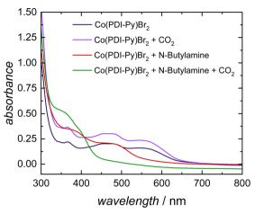
Fig. 3 Absorption measurements of 0.1 mM [Co(PDI-Pv)Br<sub>2</sub>] in MeCN solutions containing 0.03 M nBu<sub>4</sub>NPF<sub>6</sub> and 11 M H<sub>2</sub>O in N<sub>2</sub>-sparged solution (blue line), CO<sub>2</sub>-saturated solution (purple line), N<sub>2</sub>-sparged solution with 6.6 mM NBA (red line), and CO<sub>2</sub>-saturated solution with 6.6 mM NBA (green line).
