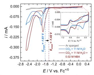
Fig. 1 Representative CVs of 0.3 mM Co(PDI-Py) in MeCN with 0.1 M  $n B u_4 N P F_6$  at a scan rate of 0.05 V s<sup>-1</sup>. CVs were taken in Ar-sparged solution (gray line),  $CO_2$ -saturated solution containing 11 M  $H_2O$  (red line), and  $CO_2$ -saturated solution containing 11 M  $H_2O$  and 0.2 M NBA (blue line). The inset is a zoom in of the region in the dashed orange box showing the  $Co^{3+/2+}$  and  $Co^{2+/+}$  peaks.
