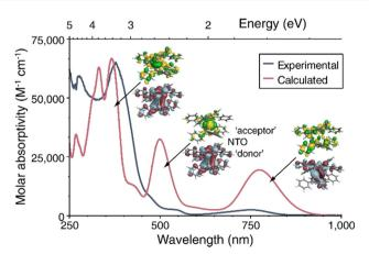
Fig. 4 UV-vis-NIR spectrum of 1-La in DME at room temperature (dark blue). TD-DFT calculated spectrum (red). Insets: representative NTOs (isosurfaces) for the most intense transitions
