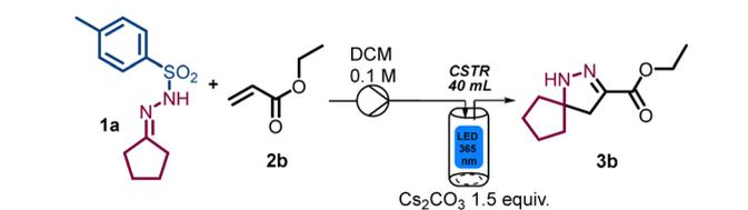
Scheme 2 Reaction scope towards spirocyclic  $\Delta^1$ -pyrazolines and  $\Delta^2$ -pyrazolines. Reaction conditions: *N*-tosylhydrazone **1a-c** (2.4 or 3 mmol), acrylate **2a-c** (2 mmol),  $\text{Cs}_2\text{CO}_3$  (2.4 or 3 mmol), DCM 0.1 M (20 mL), CSTR ( $\lambda = 365$  nm, 36.7 W or 50 W, 500 rpm), 35 °C, 20 or 30 min.
