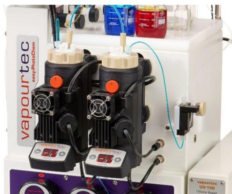
**Fig. 1** Image of photo-CSTR module with Vapourtec E-Series flow reactor.
