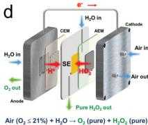
Fig. 5 Different types of setups for H<sub>2</sub>O<sub>2</sub> production. (a) One-pot setup. Reproduced from ref. 11. Copyright (2022) Elsevier. (b) H-cell. (c) Illustration of the flow cell setup. Reproduced from ref. 17. Copyright (2021) Wiley-VCH GmbH. (d) solid-electrolyte (SE) cell system. Reproduced from ref. 78. Copyright (2023) Wiley-VCH GmbH.
