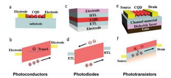
Fig. 4 Configurations of previously demonstrated CQD NIR photodetectors and their energy band diagrams. (a) and (b) Photoconductor, (c) and (d) photodiode, and (e) and (f) phototransistor. Reprinted with permission from ref. 9. Copyright 2020, John Wiley & Sons, Inc.
