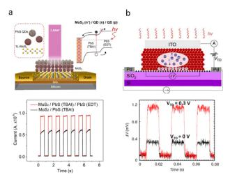
Fig. 8 (a) Device structure of the MoS<sub>2</sub>/PbS QD hybrid phototransistor and its temporal response traces. Reprinted with permission from ref. 97. Copyright 2022, American Chemical Society. (b) Device structure of the hybrid graphene-CQD phototransistor and its temporal response traces. Reprinted with permission from ref. 98. Copyright 2016, Springer Nature Limited.
