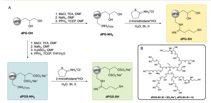
Scheme 1 Synthetic route of dPGS-SH and dPG-SH. (A) dPGS-NH2 (blue box) was synthesized in 60 g scale by mesylation, azidation, sulfation and Staudinger reduction of dPG. dPG-NH2 was synthesized similarly in small scale excluding the sulfation step. Thiolation was finally performed using 2-iminothiolane in aqueous solutions to obtain dPGS-SH (green box) and dPG-SH (yellow box). (B) Idealized schematic representation of dPGS-SH and dPG-SH.
