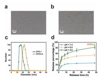
Fig. 1 Typical TEM images of DPD-1 (a) and DPDCol (b). Scale bars = 50 nm. (c) Hydrodynamic diameter distributions of DPD-1 and DPDCol. (d) *In vitro* drug release profiles of DPDMal in PBS with pH 7.4, 6.0, and 5.0 at 37 °C.
