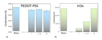
Fig. 9 Conductance at each induced pole (- and +) and among Poles after bipolar electrochemistry in phosphate buffer for (a) PEDOT:PSS and (b) IrO<sub>x</sub>. Extracted from ref. 93 under Creative Commons License.
