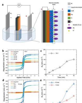
Fig. 15 CoN bipolar treatment with induction of ferromagnetism. Vertical configuration, no gradient in CoN across the field, and permanent ferromagnetism. (a) Orientation in electric field, (b and c) magnetization depending on the time of treatment. (d and e) Magnetization achieved as a function of external driving potential applied. Reproduced from ref. 105 under Creative Commons Licence.
