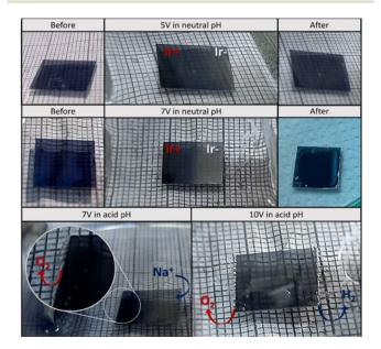
Fig. 10 Images of the IrOx coating (on Pt coated COP) acting as bipolar electrode in a phosphate buffer and acid media electrolyte and several external potentials. Reproduced from ref. 90 with permission from ACS, copyright 2021.
