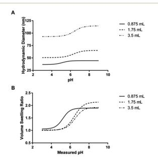
Fig. 8 Average logistic regression curves for P(AAm-co-MAA) nanoparticle swelling behavior plotted as (A) hydrodynamic diameter and (B) volume swelling ratio as a function of pH when changing the aqueous phase volume used for synthesis while keeping the organic phase volume constant (30 mL hexanes used for each formulation).
