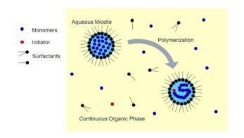
Fig. 1 Inverse emulsion polymerization scheme depicting watersoluble comonomers and crosslinker dissolved in the aqueous phase and stabilized by surfactants in the continuous organic phase. Figure adapted with permission from Zhong et al.
