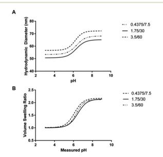
Fig. 7 Average logistic regression curves for P(AAm-co-MAA) nano-particle swelling behavior plotted as (A) hydrodynamic diameter and (B) volume swelling ratio as a function of pH when changing the overall batch volume used for synthesis. Each curve is the logistic regression fit of 3–4 independent swelling curves for each formulation. Values in the legend are reported as "aqueous phase volume/organic phase hexanes volume" (both in mL).
