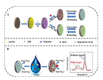
Fig. 2 Schematic of (A) MIP-based sensor construction and (B) electrochemical detection of  ${\sf HSA}^{13}$
