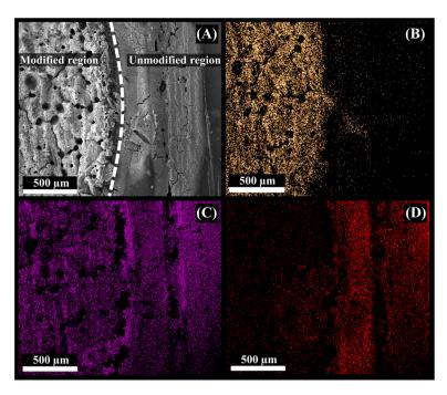
Fig. 4 (A) SEM micrograph of the modified 3D-CB/PLA electrode and colour elemental mapping images of (B) gold, (C) carbon, and (D) oxygen.
