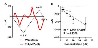
Fig. 6 Concentration curve of 5  $\mu$ M-640  $\mu$ M of Zn( $_{II}$ ) with FSCV. (A) Example "open" CV of 2.5 μM Zn(II), stars denotes reduction (\*) and oxidation (\*) peaks. (B) Concentration curve of Zn(II) with a slope of -5.164 nA  $\mu$ M<sup>-1</sup> and an  $R^2$  value of 0.9379.
