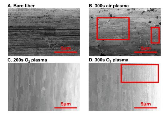
Fig. 2 SEM images of gold fibers before and after treatment. (A) An example of an untreated gold fiber. (B) A representative example of a gold fiber treated with air plasma. Surface pitting is visible. (C) An example image of a fiber treated with oxygen plasma for 200 s. (D) An example image of a fiber treated with 300 s of oxygen plasma showing pitting. Scale bars are shown on each image. Red box highlights the noted pitting observed.
