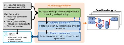
Fig. 1 The workflow of the RL-guided energy and chemical system design framework.
