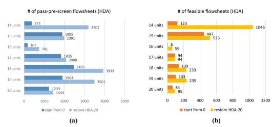
Fig. 9 RL results for HDA system with different CPPs. (a) the number of flowsheets passing pre-screen; (b) the number of feasible flowsheets.
