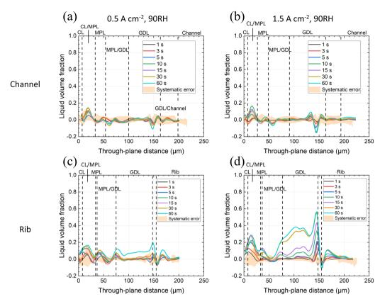
Fig. 3 Average liquid volume fraction (LVF) of product water in the CL, MPL and GDL of the *operando* VGCF-cell with 90% RH feed gases; LVF profiles are given at indicated times after the start of constant current operation with the estimated non-random error plotted as orange shade at (a) and (b) 0.5 A cm<sup>-2</sup> & 1.5 A cm<sup>-2</sup> under the channel, (c) and (d) 0.5 A cm<sup>-2</sup> & 1.5 A cm<sup>-2</sup> under the rib.
