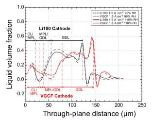
Fig. 9 LVF comparison of the Li100- and VGCF-cells at 1.5 A cm<sup>-2</sup> current density under the rib at 60 s for the RH = 90% and 110% conditions. The LVF profiles are aligned at the CL/MPL interface, and the respective domains (CL/MPL, MPL/GDL and GDL) for cells with both are specified with dashed red or black lines. Note that the thickness of the GDLs of the two cells is different, by ca. 17 µm (when uncompressed)
