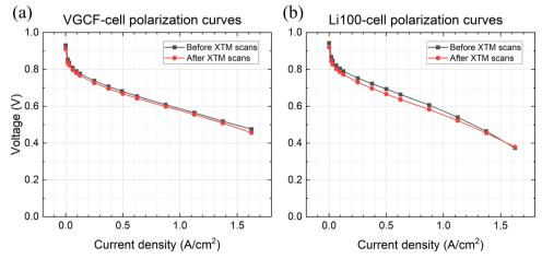
Fig. 2 Polarization curves of (a) VGCF-cell and (b) Li100-cell before X-ray exposure and after all nine tomographic scans; during polarization curve acquisition, cell temperature: 45 °C, H<sub>2</sub>/air flow rate: 200/200 mL min<sup>-1</sup>, relative humidity (RH) of H<sub>2</sub>/air: 100%/100%
