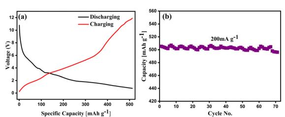
Fig. 6 (a) 12 V battery power supply at different specific capacities; (b) cycling performance of the 12 V battery at a constant current density of 200 mA g<sup>-1</sup>.
