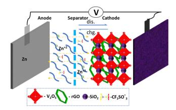
Fig. 1 Charge-discharge process with the structural alignment of the pouch cell describing the transportation of  $\mathrm{Zn}^{2+}$  ions in the presence of electrolyte with the cathode material.
