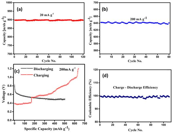
Fig. 5 Galvanostatic charge-discharge profiles at varying current densities. (a) Cycle performance at different current densities at 20 mA g<sup>-1</sup> and (b) 200 mA g<sup>-1</sup>; (c) voltage supply at different specific capacities; (d) coulombic efficiency of a single cell.
