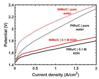
**Fig. 4** Polarization data for full HEM electrolysis using 25 wt% Ni–Mo/o-C and Pt–Ru/C (50 wt% Pt, 25 wt% Ru) cathodes using aryl-ammonium based membrane/binder polymers and IrO $_x$  anode catalysts. The total catalyst loading of Ni–Mo/oC was 1 mg<sub>cat</sub> cm $^{-2}$  and for Pt–Ru/C it was 0.15 mg<sub>cat</sub> cm $^{-2}$ . Unsupported IrO $_x$  nanoparticle anodes were loaded at 3 mg<sub>cat</sub> cm $^{-2}$ .
