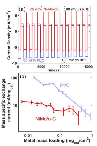
**Fig. 7** Direct comparisons of HER/HOR reversibility between Ni–Mo/oC and Pt/C catalysts. (a) Chronoamperometry measurements comprising a series of 10 minute potential steps between +100 and -100 mV vs. RHE. The mass loading of 25 wt% Ni–Mo/oC was 0.375  $mg_{cat}\ cm^{-2}$  and 60 wt% Pt/C was 0.12  $mg_{cat}\ cm^{-2}$  (b) Mass-specific exchange currents as a function of mass loading, collected from micropolarization measurements.
