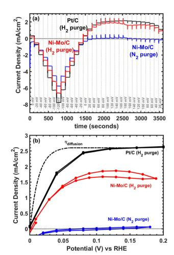
Fig. 5 Representative data for alkaline hydrogen oxidation. (a) Chronoamperometry data depicting sequential potential steps with 120 second holds used to minimize the impact of interfacial capacitance. (b) Steady-state voltammograms for Ni-Mo/oC catalyst under hydrogen and nitrogen purge compared to 60 wt% Pt/C and a simulated external transport limited overpotential curve.
