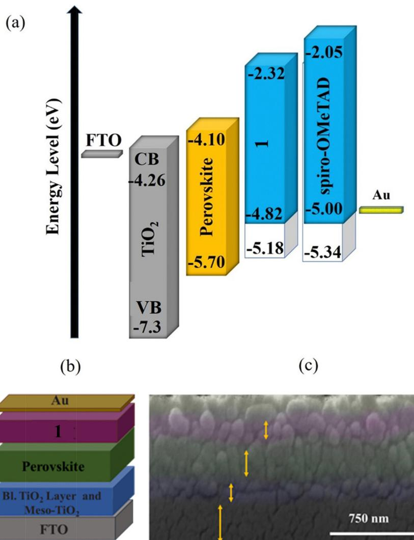
Fig. 5 (a) Diagram of energy levels of TiO<sub>2</sub>/perovskite, HTM **1** and **2** (doped/white box, un-doped/blue box), (b) device structure corresponding to the compounds applied in the investigated PSCs and (c) SEM picture of the cross-section of a demonstrative PSC based on structure FTO/TiO<sub>2</sub>/perovskite/1/Au.
