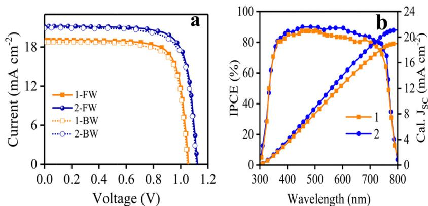
Fig. 6 The curves of (a) J–V and (b) IPCE of the devices based on HTMs **1** and **2**.
