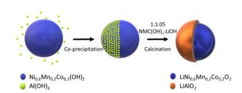
Fig. 2 Synthesis process for LiAlO<sub>2</sub>-coated Li[Ni<sub>0.6</sub>Mn<sub>0.2</sub>Co<sub>0.2</sub>]O<sub>2</sub>.
