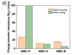
Fig. 10 Nyquist plot of NMC-P, NMC-A and NMC-B electrodes before cycling (a), and after 100 cycles (b). Column graph for the cathode electrolyte interphase resistance (c) and the charge-transfer resistance (d), before and after cycling
