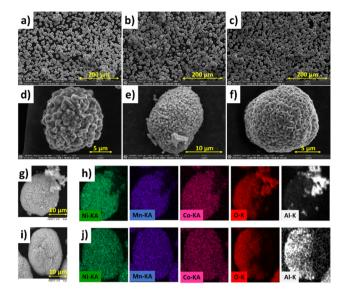
SEM micrographs of NMC-P (a and d), NMC-A (b and e) and NMC-B (c and f) at 10 kV. SEM/EDX mapping of NMC-A (g and h) and NMC-B
