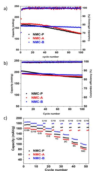
**Fig. 9** Electrochemical performance at high temperature 45  $^{\circ}$ C from 3.0 V to 4.2 V vs. Li<sup>+</sup>/Li (a), at room temperature and high potential window from 3.0 to 4.4 V vs. Li<sup>+</sup>/Li (b). Rate capability (c).
