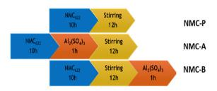
Fig. 1 Synthesis process for different Al(OH) $_3$ -coated Ni $_{0.6}$ Mn $_{0.2}$ -Co $_{0.2}$ (OH) $_2$  precursor samples.
