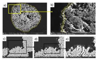
Fig. 5 SEM of a cross-sectioned NMC-B particle (a), the dotted lines represent the LiAlO<sub>2</sub> coating layer. The framed region shows a zoom on the LiAlO<sub>2</sub> coating layer (b). Cross-section of another NMC-B particle (c). The framed region shows a zoom on the LiAlO<sub>2</sub> coating layer (d and e).
