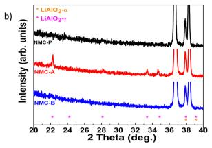
Fig. 3 XRD patterns of NMC-P, NMC-A and NMC-B (a), and the zoom plot of the region showing the main LiAlO<sub>2</sub> peaks (b)
