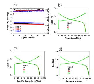
Fig. 8 Electrochemical performances of various samples at room temperature from 3.0 V to 4.2 V vs. Li<sup>+</sup>/Li (a). Charge/discharge curves for NMC-P (b), NMC-A (c) and NMC-B (d).
