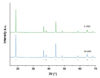
Fig. 2 XRD pattern of SS-LNO synthesised at 700  $^{\circ}$ C for 12 hours in O<sub>2</sub> (blue), and C-LNO synthesised at 800  $^{\circ}$ C for 1 hour in O<sub>2</sub> (green).
