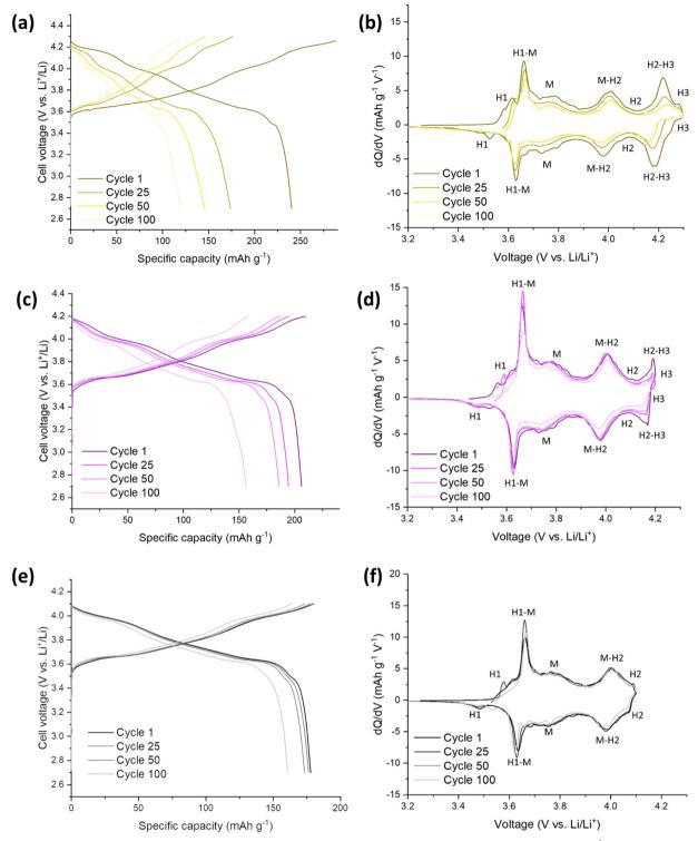
Fig. 6 Electrochemical performance during galvanostatic charge and discharge of Mo-LNO/Li half cells at 10 mA  $g^{-1}$ : (a) between 2.7-4.3 V (b) corresponding differential capacity (dQ/dV) plot with phases (c) between 2.7-4.2 V (d) corresponding differential capacity (dQ/dV) plot with phases (e) between 2.7-4.1 V (f) corresponding differential capacity (dQ/dV) plot with phases.
