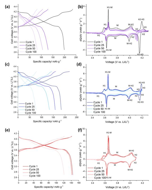
Fig. 3 Electrochemical performance during galvanostatic charge and discharge of SS-LNO/Li half cells at 10 mA g<sup>-1</sup>: (a) between 2.7-4.3 V (b) corresponding differential capacity (dQ/dV) plot with phases (c) between 2.7-4.2 V (d) corresponding differential capacity (dQ/dV) plot with phases (e) between 2.7-4.1 V (f) corresponding differential capacity (dQ/dV) plot with phases.
