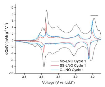
Fig. 4 Comparison of first cycle differential capacity (dQ/dV) plots for Mo-LNO (black), SS-LNO (red) and C-LNO (blue) in the voltage window 2.7-4.3 V. This shows a shift to a higher voltage for the H2-H3 phase transition in Mo-LNO
