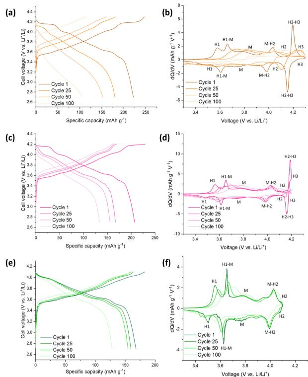
Fig. 5 Electrochemical performance during galvanostatic charge and discharge of C-LNO/Li half cells at 10 mA g<sup>-1</sup>: (a) between 2.7-4.3 V (b) corresponding differential capacity (dQ/dV) plot with phases (c) between 2.7-4.2 V (d) corresponding differential capacity (dQ/dV) plot with phases (e) between 2.7-4.1 V (f) corresponding differential capacity (dQ/dV) plot with phases.
