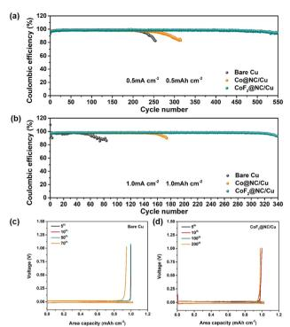
Fig. 3 Coulombic efficiency of the Li|Cu cells with CoF2@NC/Cu, Co@NC/Cu and bare Cu substrates at (a) 0.5 mA cm<sup>-2</sup> and (b) 1 mA cm<sup>-2</sup> for 1 mA h cm<sup>-2</sup>. Voltage profiles of the Li|Cu cells with (c) CoF<sub>2</sub>@NC/Cu, (d) Co@NC/Cu, and (e) bare Cu current collectors at 1 mA cm<sup>-2</sup> and  $1 \text{ mA h cm}^{-2}$
