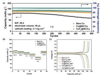
Fig. 8 Electrochemical performance of LFP full cells with CoF2@NC/Cu, Co@NC/Cu, and bare Cu current collectors. (a) Cycling stability of the full cells at the rate of 1C, (b) rate performance of the full cells, and (c) voltage profiles of the full cells at the 1st and 200th cycles
