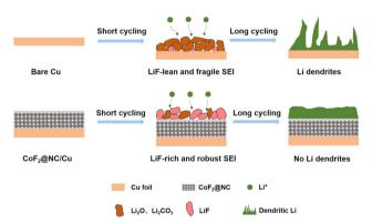
Fig. 7 Schematic illustration of the Li stripping/plating cycling on (a) bare Cu and (b) CoF2@NC/Cu current collectors.
