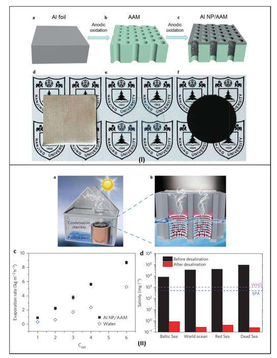
Fig. 7 Plasmonic-based water purification SIWE devices; (I) fabrication process of the Al NP-based plasmonic structure and (II) (a) and b) set-up and schematic of plasmon-enhanced solar desalination, (c and d) performances based on mass change and evaporation rate achieved, respectively. Reproduced with permission.<sup>8</sup> Copyright 2016, Springer Nature.
