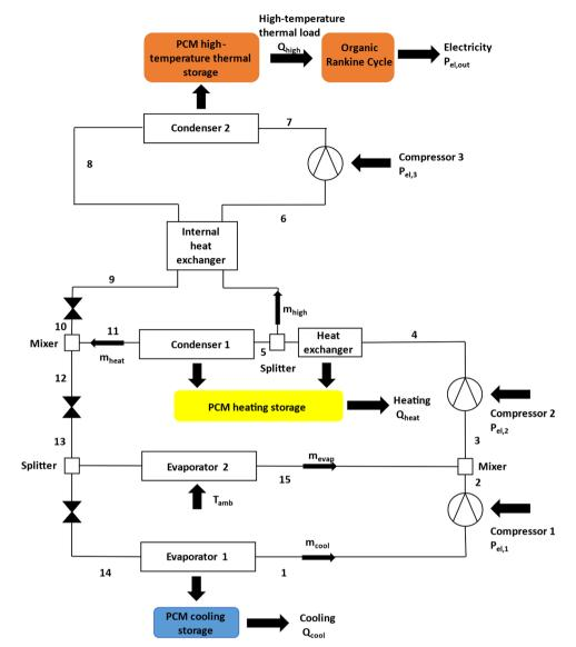
Pumped thermal energy storage unit for building trigeneration.
