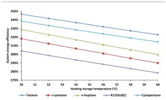
Fig. 6 Overall energy efficiency depending on the heating storage
