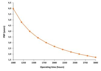
Fig. 12 Payback period for different system operating hours.
