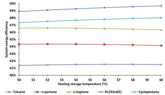
Overall exergy efficiency depending on the heating storage temperature
