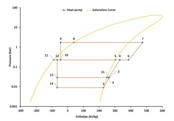
Fig. 11 Heat pump pressure–specific enthalpy (P-h) diagram.
