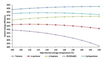
Fig. 5 Overall exergy efficiency depending on the high-thermal storage temperature
