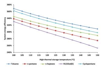
Fig. 4 Overall energy efficiency depending on the high-thermal storage temperature
