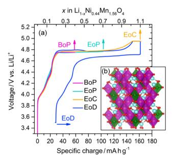
Fig. 1 (a)  $Li_{1-x}Ni_{0.44}Mn_{1.56}O_4$  charge-discharge profile obtained from the partial curves of the individual cathodes from different states of charge (see text for the definitions): BoP, EoP, EoC, and EoD, respectively. The inset (b) shows the spinel crystal structure in the cation ordered P4332 space group of LiNi<sub>0.5</sub>Mn<sub>1.5</sub>O<sub>4</sub>; Li (blue), O (red), Ni (green), and Mn (purple).<sup>21</sup>
