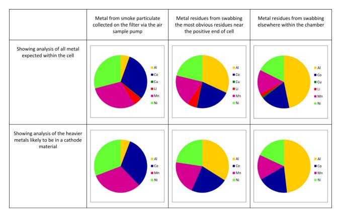
Fig. 6 Proportions of metals observed from samples taken from failure of cell C.
