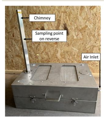
Fig. 1 Test Enclosure
