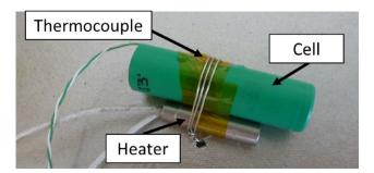
Fig. 2 A cell prepared for testing
