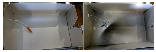
Fig. 5 The test chamber before and after a test.
