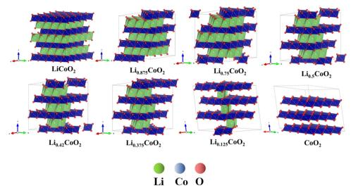
Fig. 6 The phase transformation of  $\text{Li}_x\text{CoO}_2$  during delithiation: the  $\text{Li}_x\text{CoO}_2$  evolves from the O3 phase to the O1 phase and the gradual angle keeps decreasing during delithiation.48
