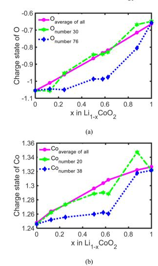
Fig. 5 The average charge states of all O, individual O<sub>number 30</sub> with surrounded Li extracted, and individual Onumber 76 without surrounded Li extracted in LixCoO2 during delithiation (a); the average charge states of all Co, individual Co<sub>number 20</sub>, and individual Co<sub>number 38</sub> in Li<sub>x</sub>CoO<sub>2</sub> during delithiation (b)
