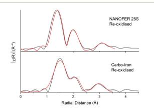
Fig. 3 U L<sub>3</sub>-edge Fourier transform data (black) and fits (red) for the re-oxidised NanoFeR25s and Carbo-Iron samples.
