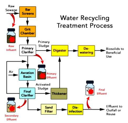
Steven M. Clouse WRC activated sludge treatment process stages and sample collection points.
