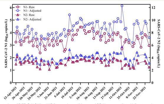
Fig. 2 Concentrations of SARS-CoV-2 N1 and N2 (log<sub>10</sub> copies per L) in raw and BCoV recovery adjusted influent samples.
