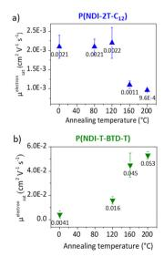
Fig. 4 (a) and (b) Electron mobility in saturation regime ( $V_{\rm DS}$  = +100 V) as a function of the annealing temperature of P(NDI-2T-C<sub>12</sub>) and P(NDI-T-BTD-T) bottom gate bottom contacts OFETs.
