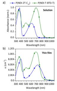
Fig. 2 UV-Vis absorption spectra of both polymers (a) in chlorobenzene solution at 298 K normalized to the maximum absorption peak, and (b) as as-cast thin films in ambient conditions.
