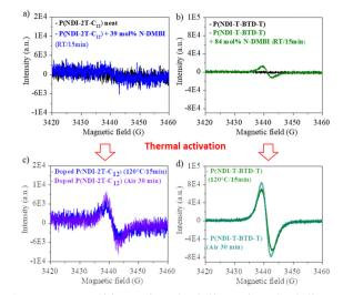
Fig. 5 EPR spectra of (a) neat P(NDI-2T-C12) and P(NDI-2T-C12):N-DMBI mixed at RT in toluene (inert atmosphere, in dark), (b) Neat P(NDI-T-BTD-T) and P(NDI-T-RTD-T):N-DMRI mixed at RT in chlorobenzene (inert atmosphere, dark). (c) and (d) Same solutions heated up at 120 °C in inert atmosphere and exposed to air. Magnetic field power: 158.63 mW, modulation amplitude: 3.0 G
